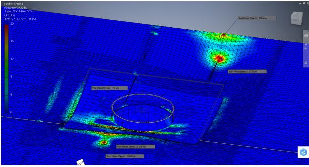
Pictured below, as requested, Von Mises Stress view of main deck (48"x48" main deck doubler hidden):
