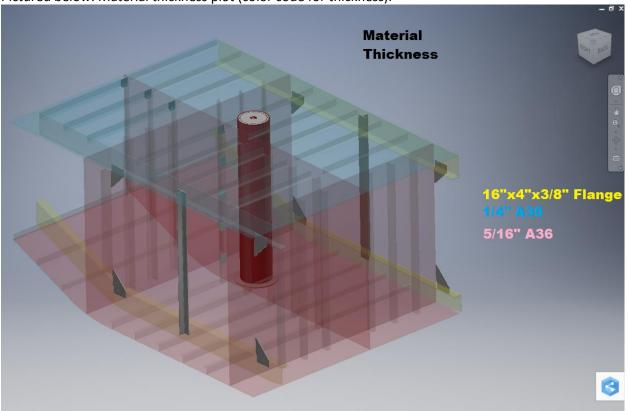
Pictured below: Material thickness plot (color code for thickness).
