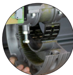
CROWN WHEEL MOUNTED ON ROLLER BEARINGS
