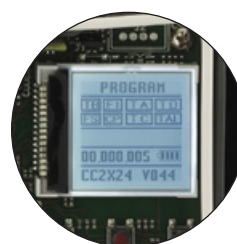
SELF-PROGRAMMING MONITORED BY AN LCD GRAPHICS DISPLAY
