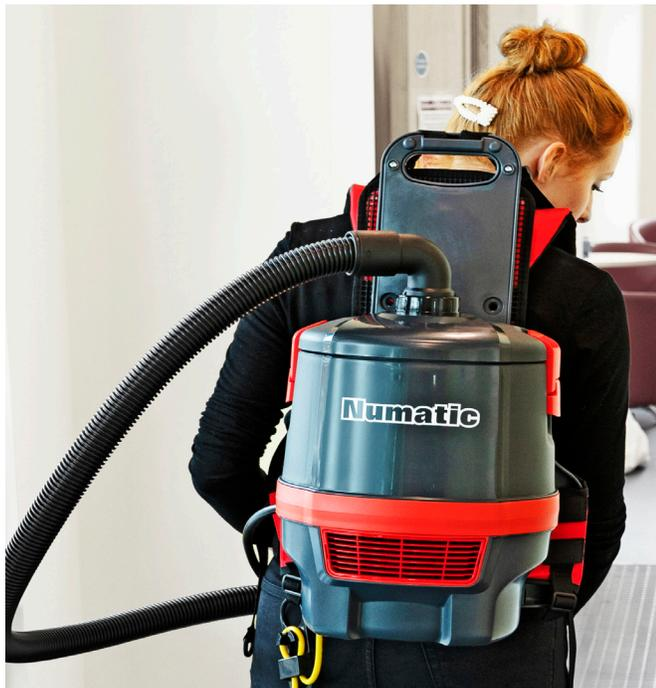
The adjustable back support, waist and shoulder straps are designed to minimize operator fatigue and the hose features swivel fittings to ensure tangle-free operation. This unit is equipped with a four-stage filtration system providing 0.3-micron filtration at 99.97% efficiency, improving indoor air quality and reducing dust in the building.
