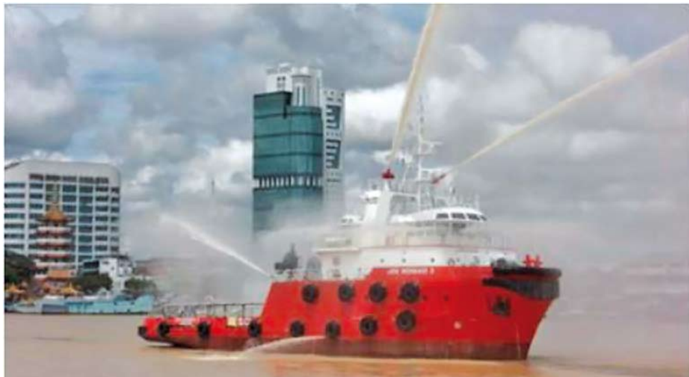
Anchor Handling Tug Testing Fire-fighting equipment during the Official Trial
