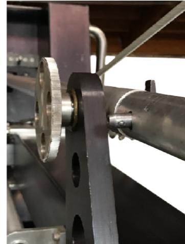
Leveling Mechanism Turnbuckle
