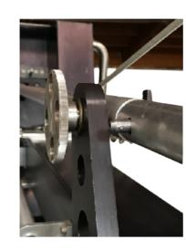
Leveling Mechanism Turnbuckle
