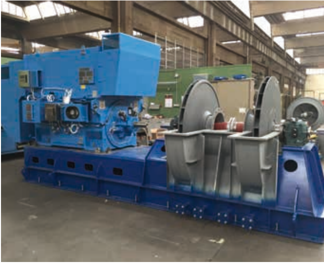
SRU UNIT - COMBUSTION AIR BLOWER
