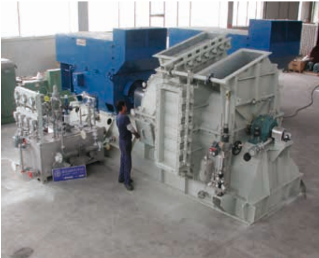
UREA PLANT - ATOMIZATION AIR BLOWER
