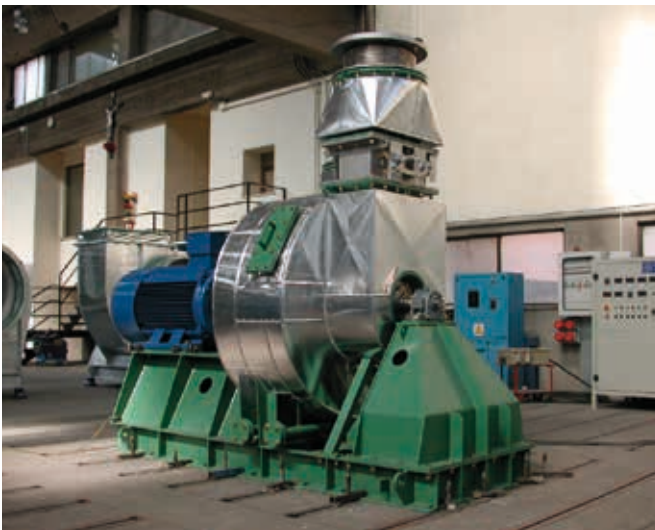
COKE OVEN GAS BLOWER
