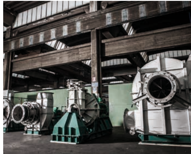
BLOWER SET FOR FORMALDEHYDE PLANT
