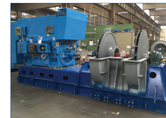
◆ FORMALDEYDE GAS BLOWER
