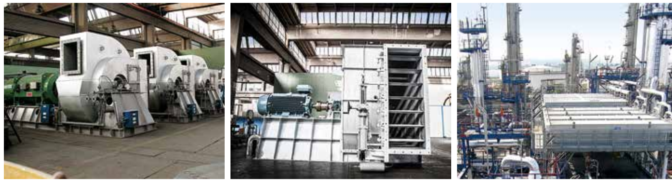
INCINER. AIR BLOWER - SRU FLUEGAS FAN - H2 FURNACES AUTO OIL 2 - REFINERY
