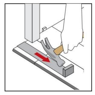
**15. Place and Secure Row End Planks** Ensure end joint at end of last plank of the row is completely engaged, using a pull tool.
