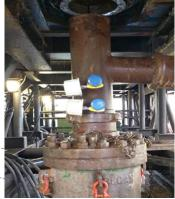
Bell Nipple Sensor (can use one or both Density @BN probes)
