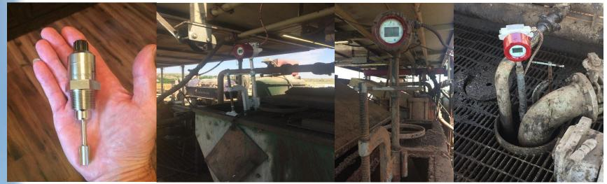
Resonant Freq and Damping Detectors - mud density & viscosity; recent (2018Q2) successful deployment in Texas, accuracy @ 0.5% and very repeatable.
