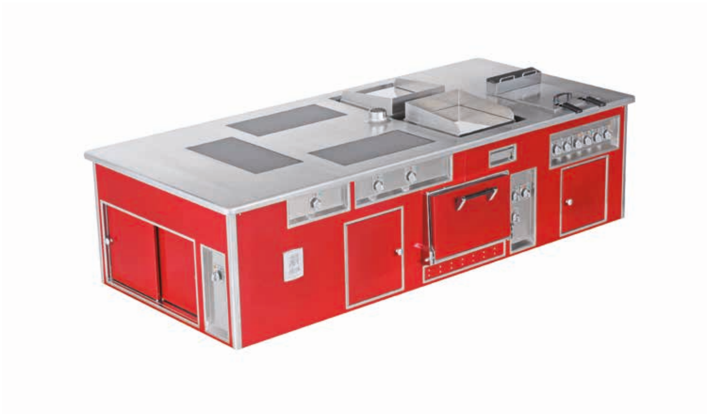
Traditional made to measure central stove, red enamelled finish, stainless steel and chromium trims, 3 induction plates, 2 electric chromed smooth grills, electric fryer, 2 electric ovens GN 2/1, hot cupboard.
