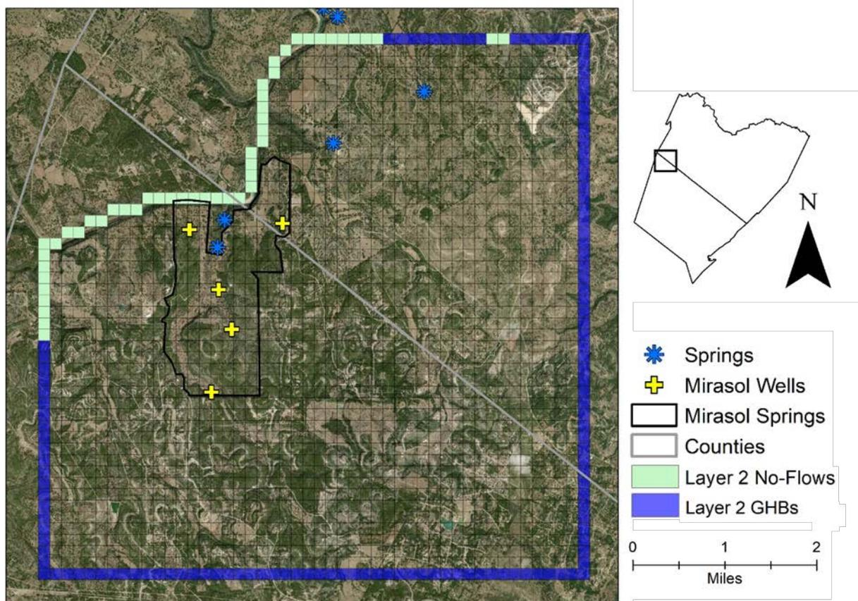
**Figure 8. GHBs and no-flow boundaries in Layer 2. All boundaries in Layer 1 are no-flows.**
