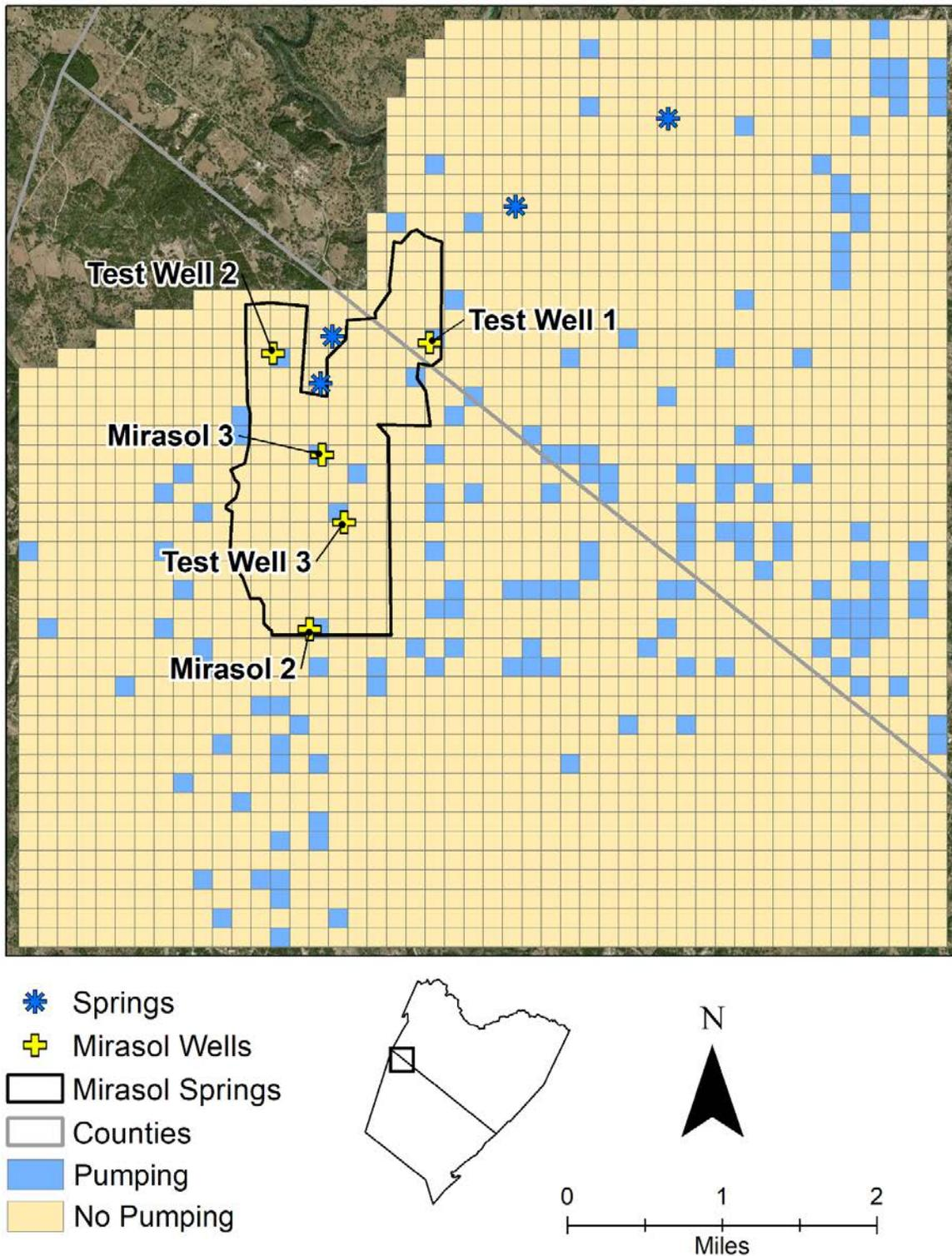
Figure 11. Cells where pumping is applied, including the proposed Mirasol Wells.
