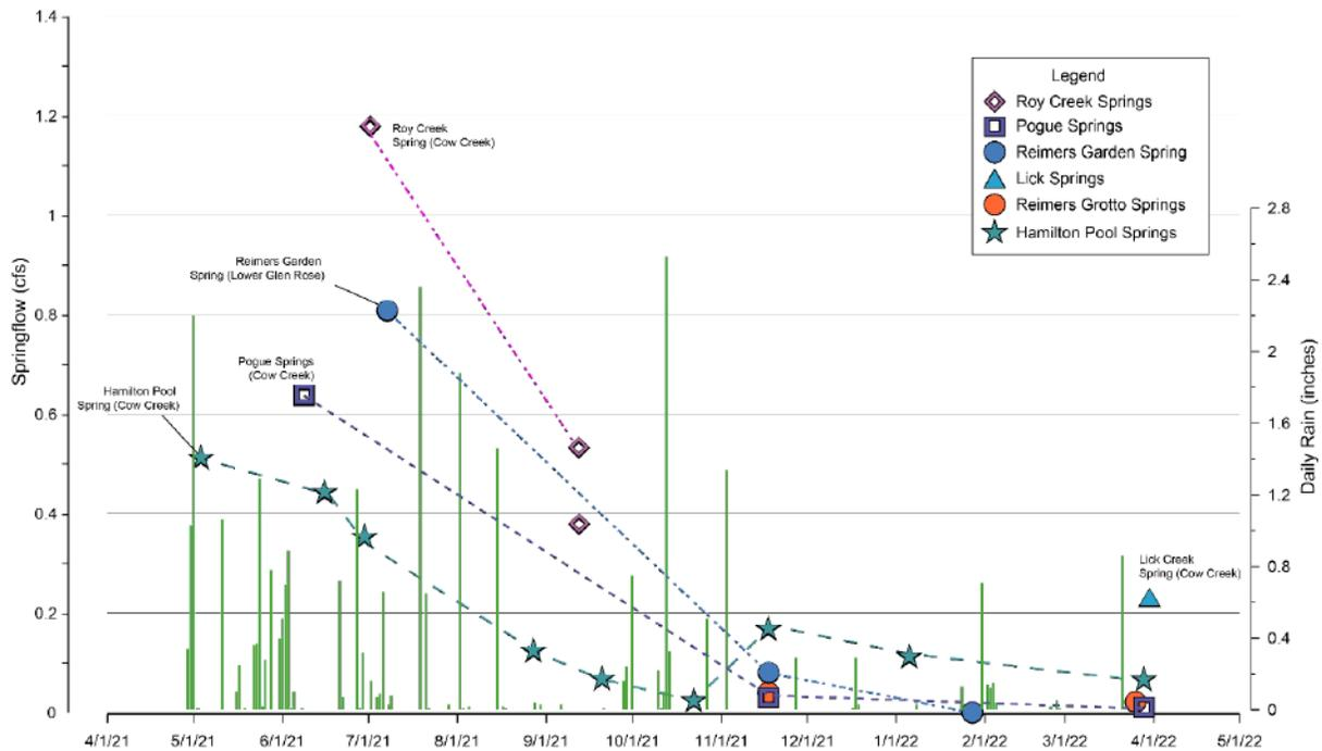
Figure 5. BEG figure detailing rainfall data overlain with spring flow measurements in the study area.
