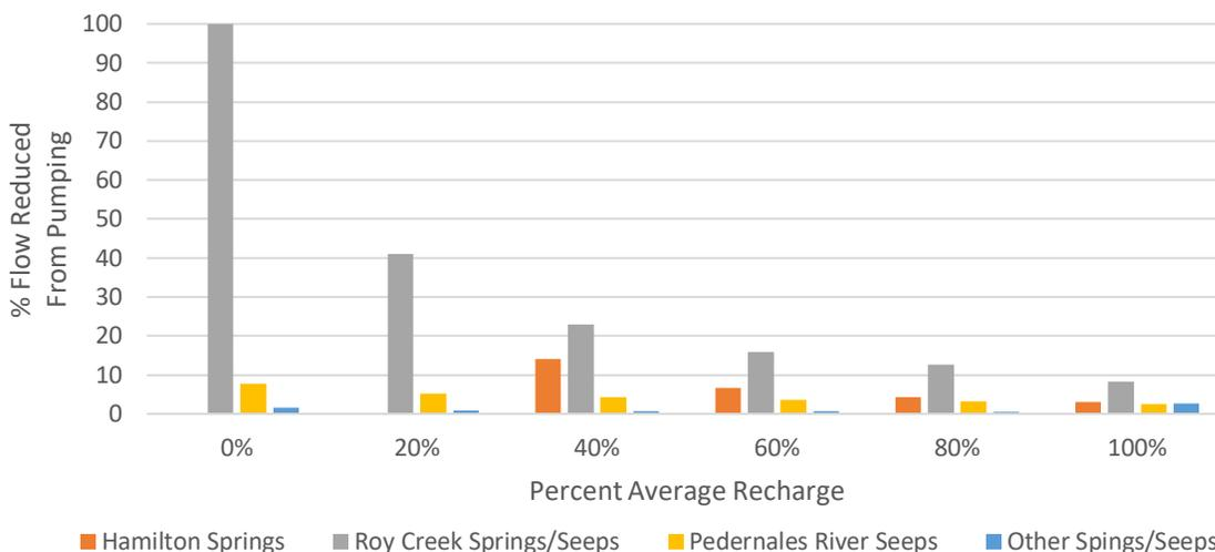
**Figure 18.** Percent of baseline flow reduced by simulated mirasol pumping in different recharge conditions.
