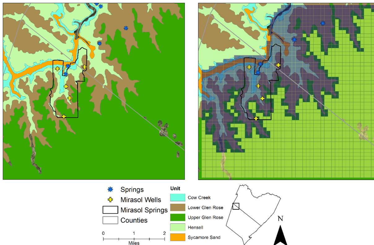
Figure 9. Texas GAT in our study area. Cells with recharge applied are shaded in blue.
