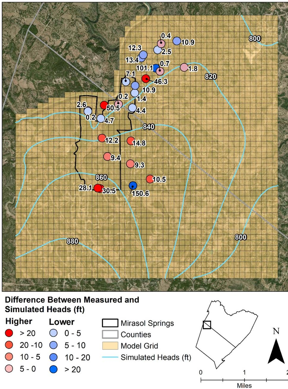
Figure 12. Simulated water levels and difference from observed values.
