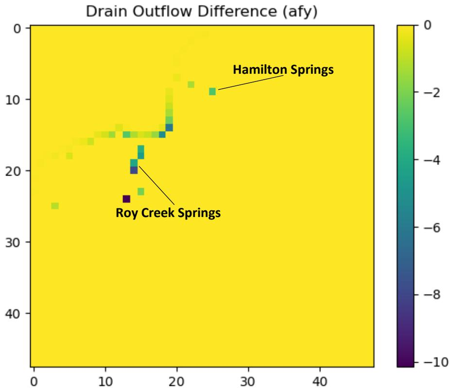
Figure 15. Spatial distribution of the reduction of drain discharge (acre-feet per year) due to the proposed Mirasol production wells during average rainfall conditions.
