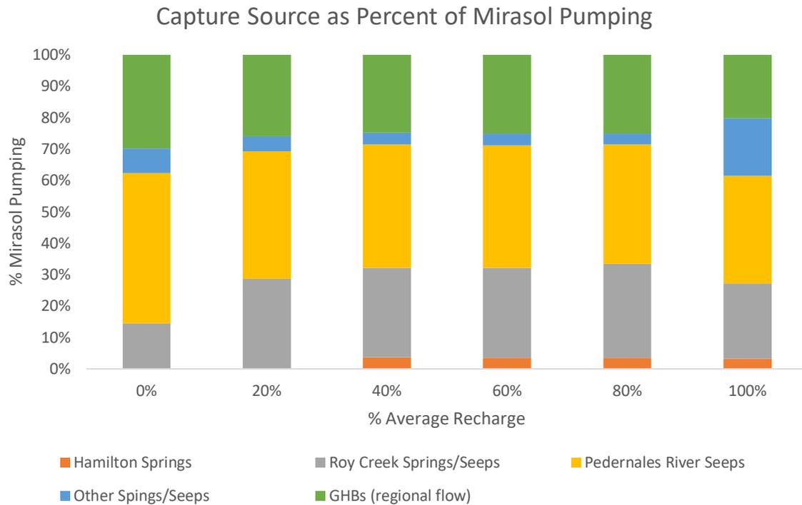
Figure 16. Flow volume reduced from each source or sink (“capture”) expressed as a percent of Mirasol pumping for the range of recharge volumes analyzed.
