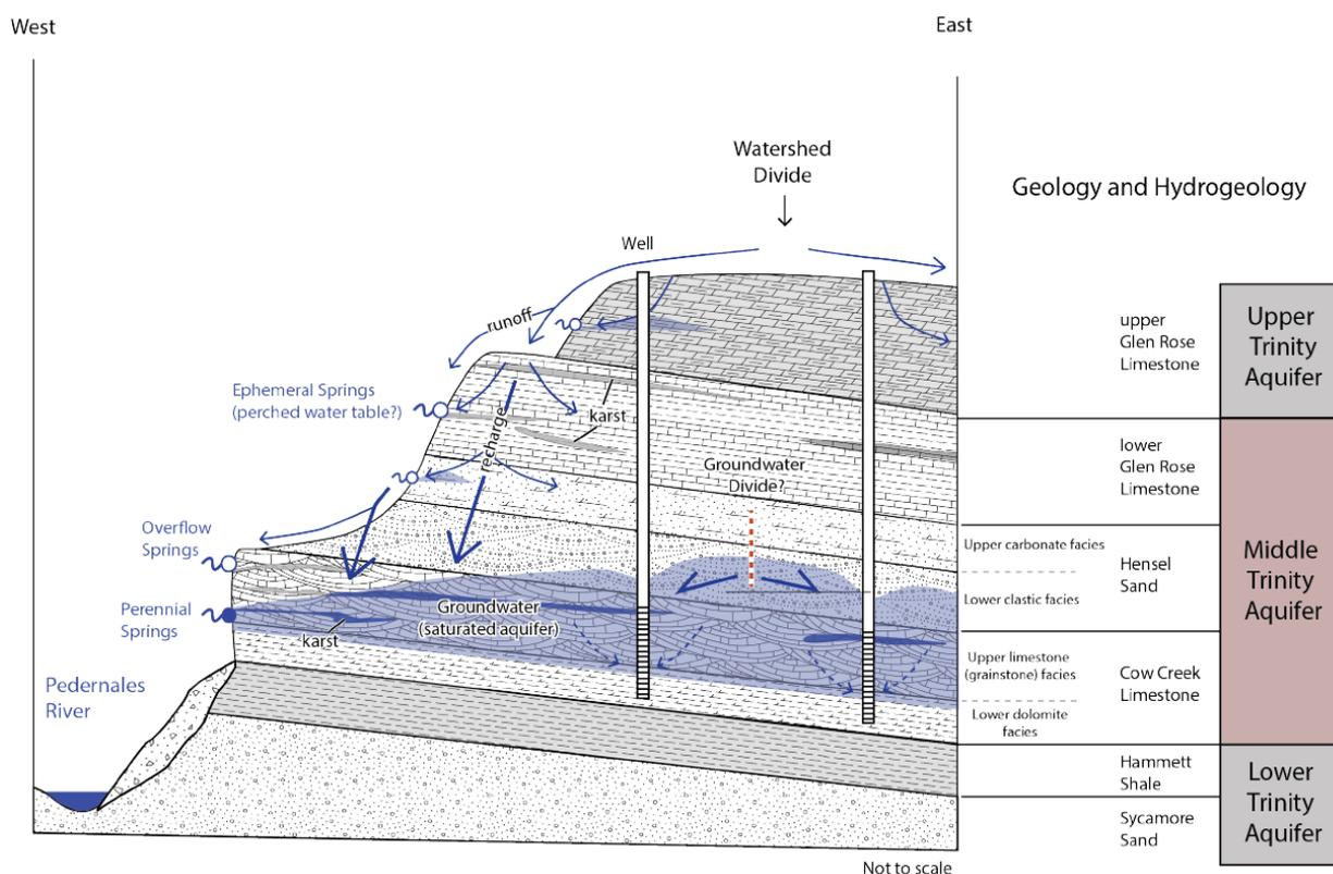
Figure 3. Conceptual hydrogeologic framework (Hunt, 2022)
