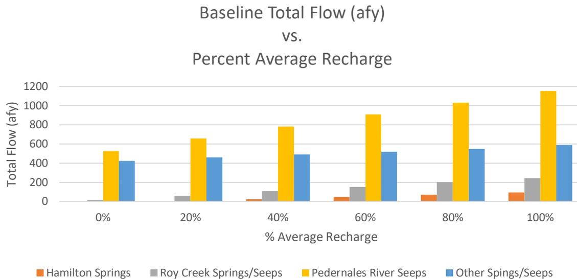
Figure 17. Flow volumes from each analyzed spring or seep before the addition of Mirasol Pumping for the range of recharge volumes analyzed.
