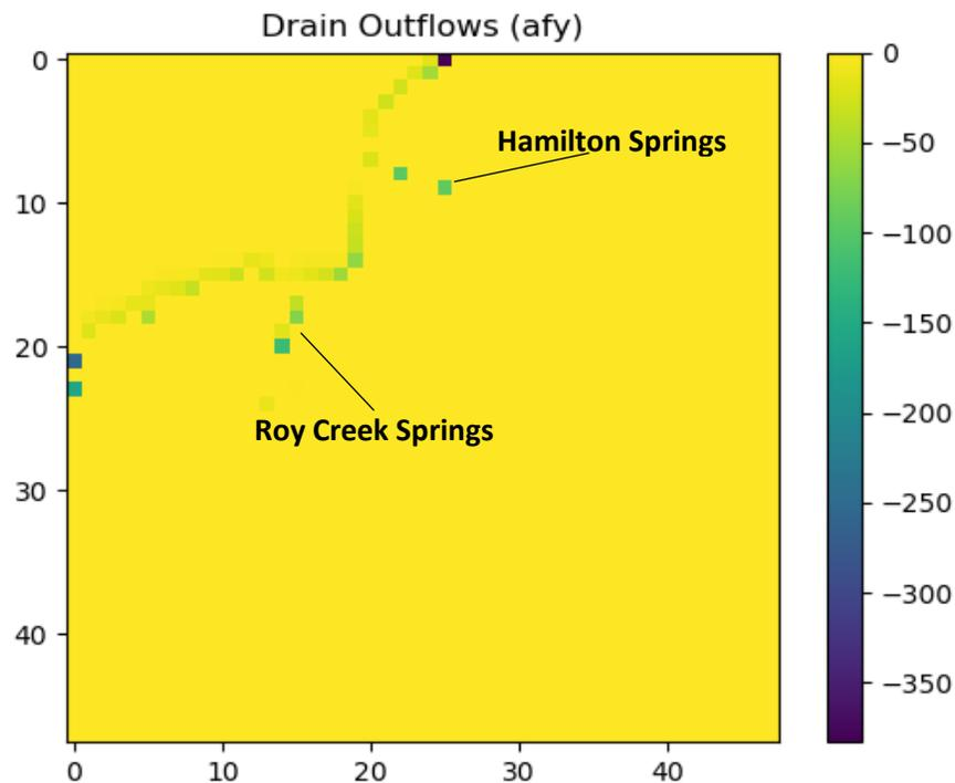
**Figure 14.** Spatial distribution of springs and seeps outflow in the calibrated model.
