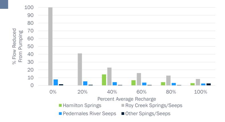
The volume of capture for each source/sink remains relatively constant, though the capture expressed as a proportion of the baseline flow increases as recharge decreases
