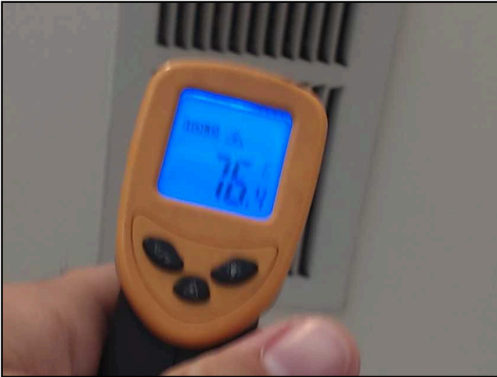
The second floor AC unit did not appear to adequately cool when tested.
