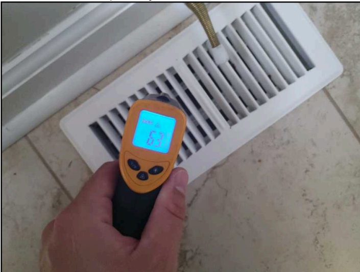
There was a 14 degree temperature differential when the air conditioning was tested at the main floor level when tested.
