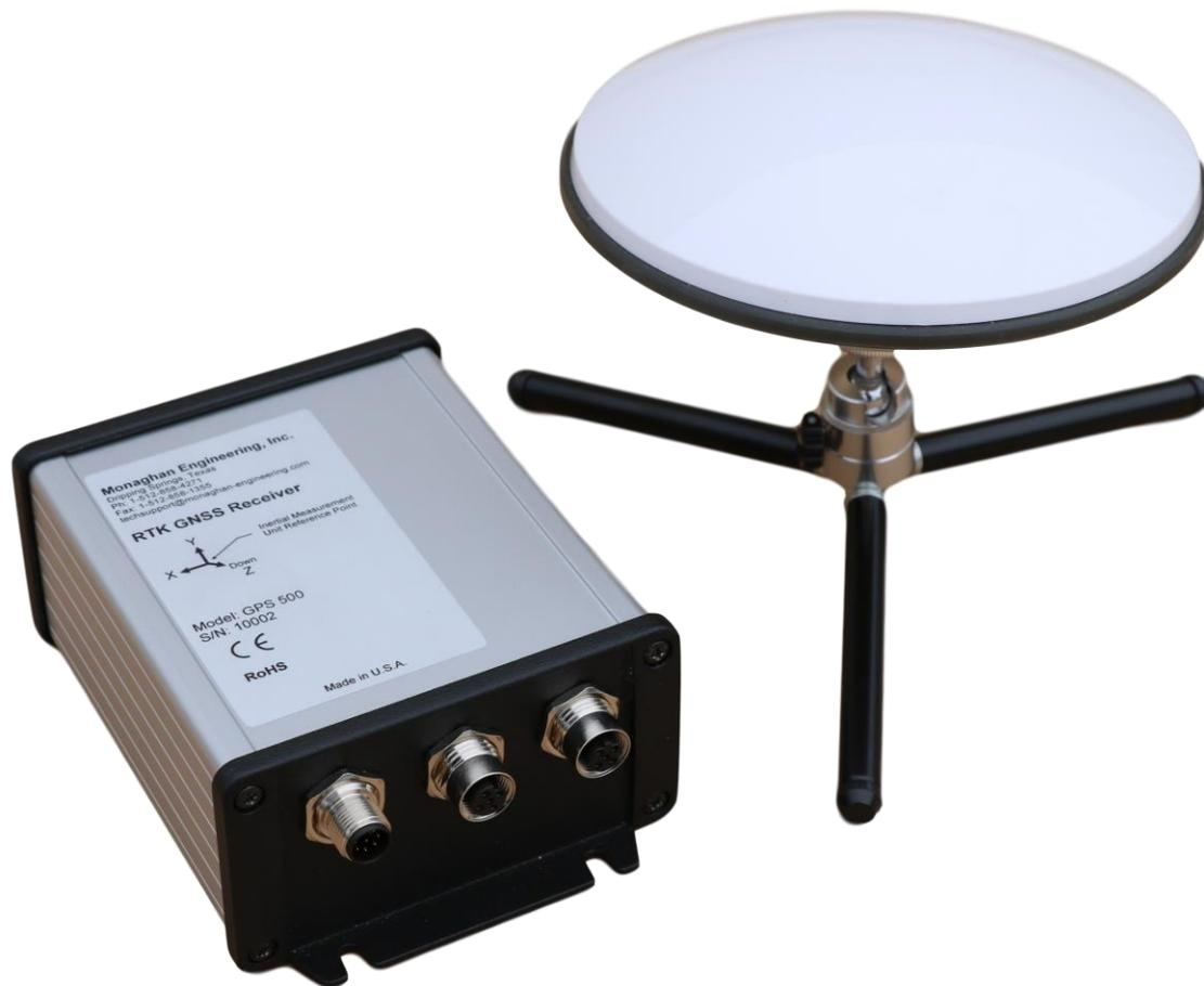
The GPS 500 provides a direct communications interface to the PME GPS 0100 Network Time Server module to allow an M580 Controller access to precise time and position information. It provides 2 cm position accuracy and a 1 Pulse per Second output accurate to +/- 60 nS.
