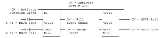
Once the event buffer is full, or the time delay after putting an event in the buffer is up, the top output is turned ON in order to activate the MSTR function block. The top output remains ON until the MSTR function block feeds back a transmission completion through the middle input.
