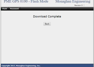
The PME GPS 0100 can be returned to operating mode by power cycling the module or by inserting a paper clip through the Setup hole until the front panel lights stop flashing, approximately 5 seconds.
