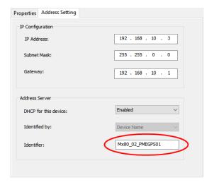
In this example, the PME GPS 0100 is located in the CPU rack, Slot 2. Therefore, the Identifier must be set for "Mx80\_02\_PMEGPS01". The following are the valid entries for the Identifier.
