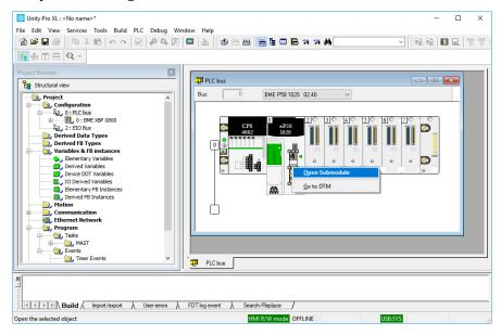
The FTP server must be enabled tin the PLC for any PME module to function. The easy way to enable the server is to select "Unlock Security".
