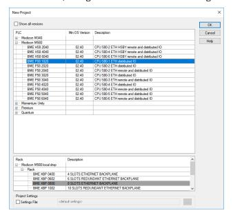
After selecting the "PLC Bus" in the Structured View Tree, right click on the Ethernet ports of the CPU to open the configuration submodule.
