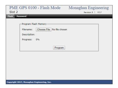
Click the "Choose File" button to select the firmware image to load. Click "Program" to start the programming process. The front panel LED's will stop flashing for approximately 5 seconds while the Flash memory is erased. The program description will then be displayed and the Progress indicator will show the percentage complete.
