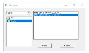
A File Open screen will appear. Select the new PME GPS 0100 XML DTM file.
