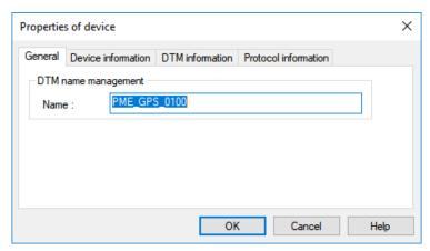
Pressing "OK" will add the DTM device to the DTM Browser. The PME GPS 0100 is now added to the tree below the PLC.
