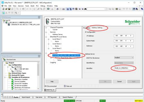
The "Identifier" must be modified to define the exact Rack and Slot occupied by the PME GPS 0100 module.
