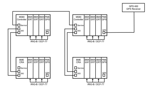
The PME GPS 0100 communicates across the ethernet backplane. For modules located in different racks, the module operating as a time server communicates with modules operating as clients through the ethernet ring connecting the racks. The typical error between modules located in different racks is less than 1 microsecond.
