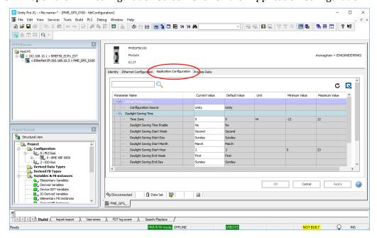
This screen is used to configure the parameters that are downloaded to the PME GPS 0100 at startup. Most of the selections are enumerated values that are selected by a drop-down menu. They are organized in groups by function.
