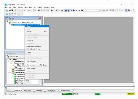
This will open the DTM configuration screen. Click on the "Application Configuration" Tab.
