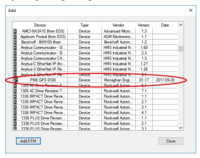
Highlight the PME GPS 0100 entry and press Enter or "Add DTM" to load the DTM for the PME GPS 0100 module. A window will pop up with information about the DTM.
