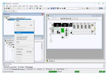
If the connection is successful you will be able to select: Device Menu>Additional Functions>Reset Device.
