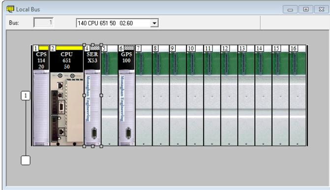
Double clicking the SERx53 00 card will bring up the configuration screen where you can enter the proper starting addresses for the card.
