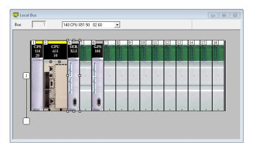
Double clicking the cards will bring up the configuration screen where you can enter the proper starting addresses for each card.
