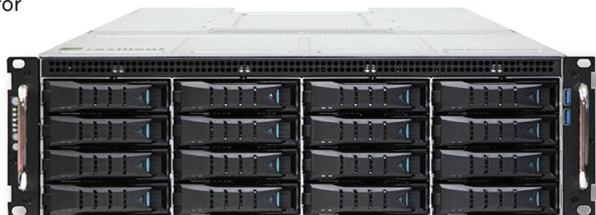
This standalone 3U rack mountable fully redundant appliance has three different versions to support from 50 camera streams to 300 camera streams. iCentana's analytics is preloaded into the system. It has dual Intel Xeon processors and multiple Nvidia GPUs depending on the number of camera streams. Up to 54TB of usable HD storage is included for storage with RAID 6 for data integrity.
