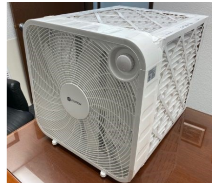
A Corsi box (pictured) is a low-cost, DIY indoor air filtration solution that consists of one box fan plus five filters arranged in a cube. COURTESY OF TEX-AIR FILTERS
