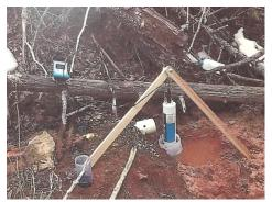
Figure 4: Hydrolab testing water in Swift Gulch
