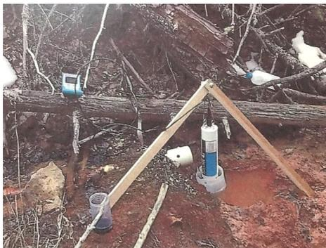
Figure 4: Hydrolab testing water in Swift Gulch
