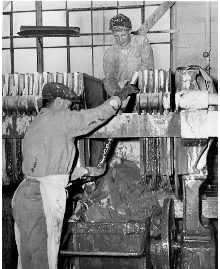
ACM employee Bill Linn, standing above, recovers leach material from an overflow tank in 1955
