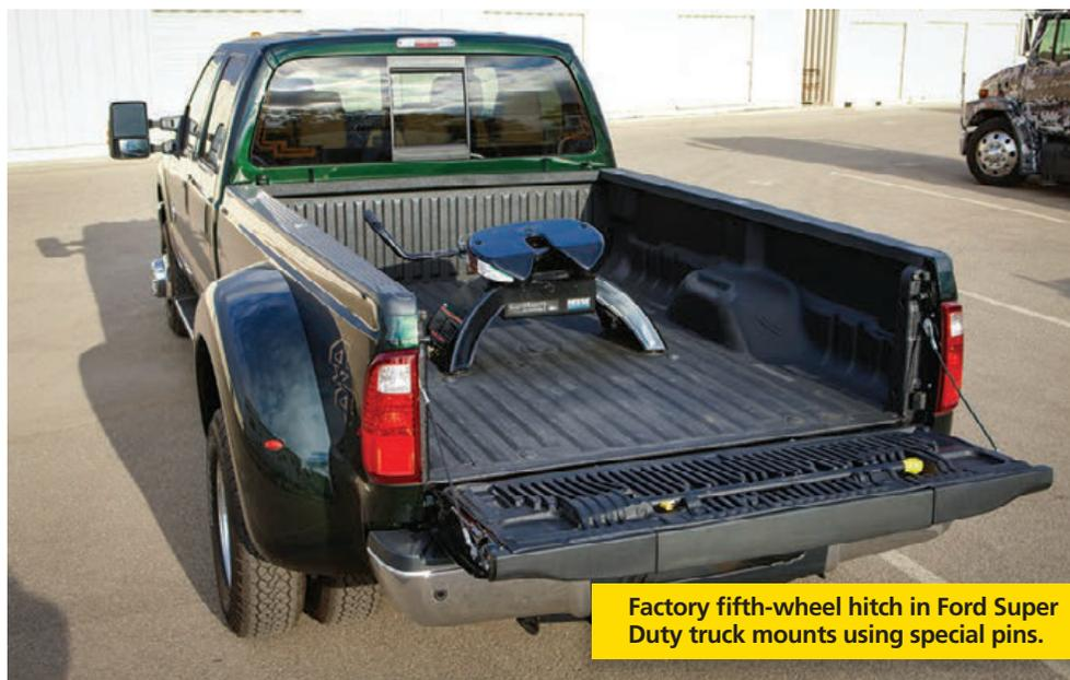
**Factory fifth-wheel hitch in Ford Super Duty truck mounts using special pins.**
