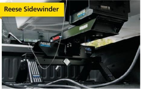
than ever, particularly among extended-cab models. However, a shortbed often causes complications when using the truck for towing a fifth-wheel because the proper hitch-mounting location is far enough forward to cause trailer-to-cab collisions during sharp turns. Installing an extended pinbox provides a workable solution with smaller trailers with modest pin weights; however, owners should first check with the pinbox manufacturer before adding any extension.
