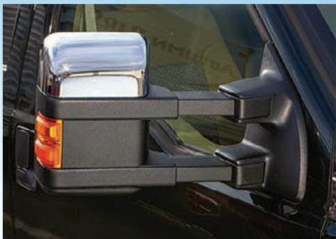
Ford's towing mirrors easily extend for optimum visibility of the trailer — superior to add-on mirrors.
