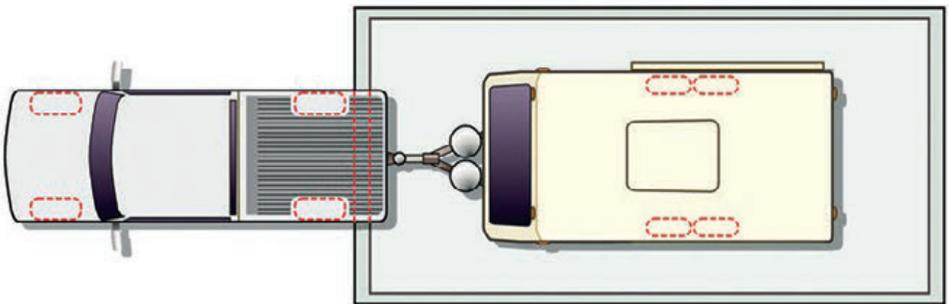
**To determine weight, first get a reading on axle weight, then unhitch the trailer for a total weight reading (with the tow vehicle's wheels off the scale), and then subtract the two.**
