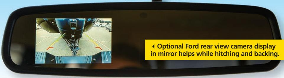
◀ Optional Ford rear view camera display in mirror helps while hitching and backing.
