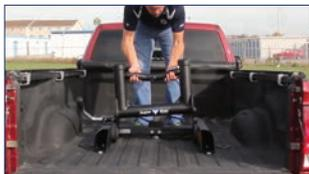
**Slide the shock towers into the base.**
