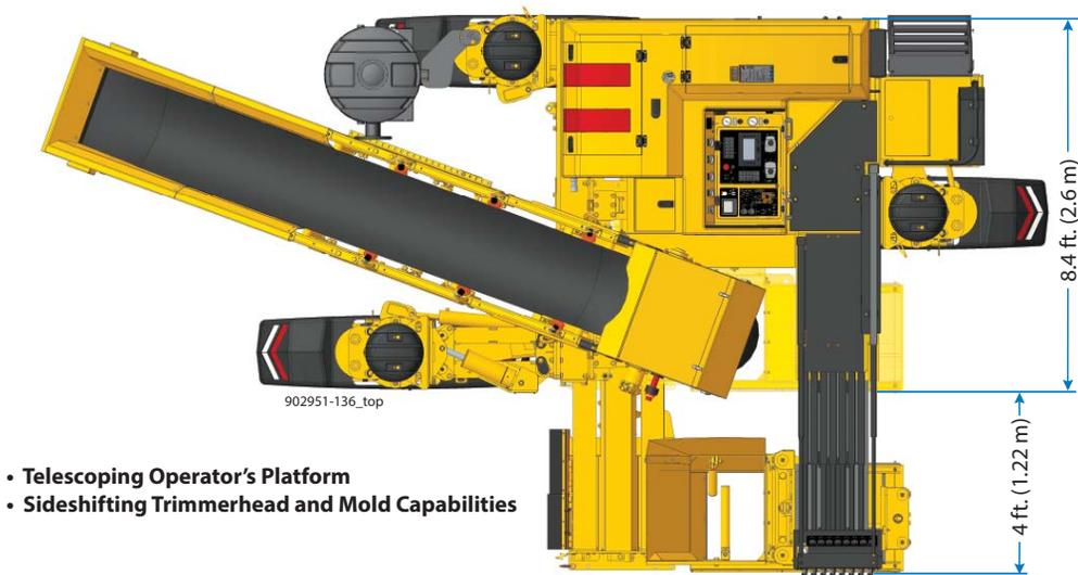
**All-Track Positioning (ATP)** provides the versatility in our slipform pavers. GOMACO's left-front track features a pivoting power-swing, the right-front track hydraulically extends/retracts, and the rear track hydraulically sideshifts. Each leg has a reinforced steel attachment plate that allows extra leg height adjustment. ATP provides the capability of performing various applications and working with differences in grade elevations and unique job-site logistics.
