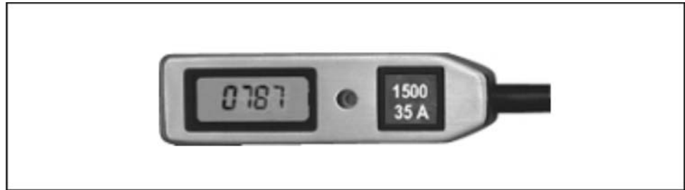
Figure 3-16. Example of Military CYPRES Control Unit Setting
