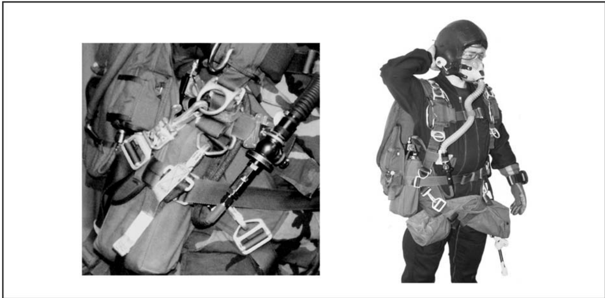
Figure 4-7. Completed Rigging of the Portable Bailout Oxygen System With the AIROX VIII Assembly to the RAPS
