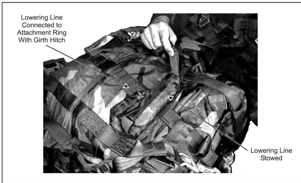
Figure 5-40. Lowering Line Attached to the Attachment Ring on the Drop Bag With a Girth Hitch or a Locking Carabiner
