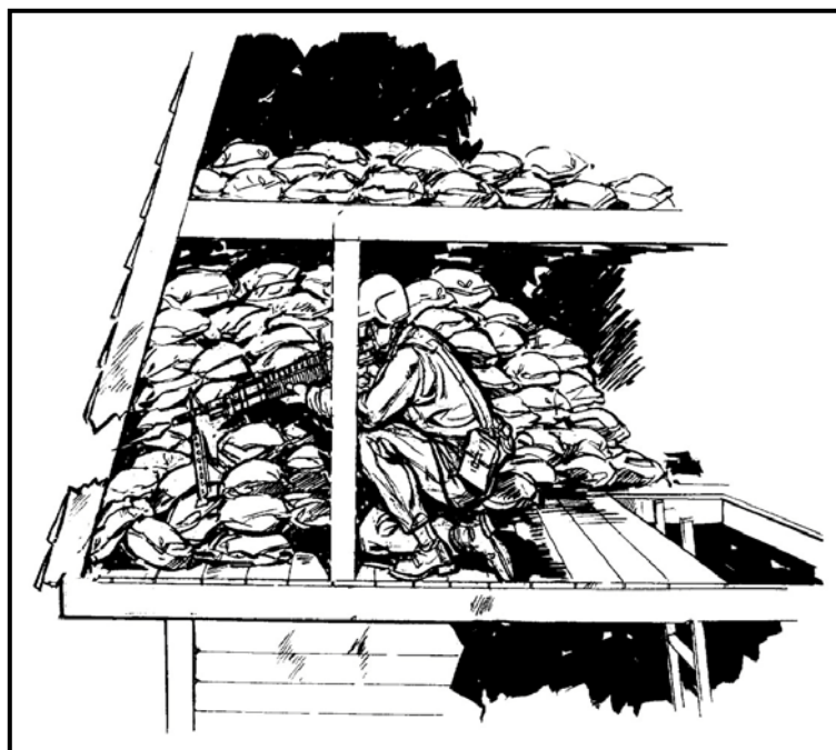
Figure 3-60. Firing platform built under roof.
