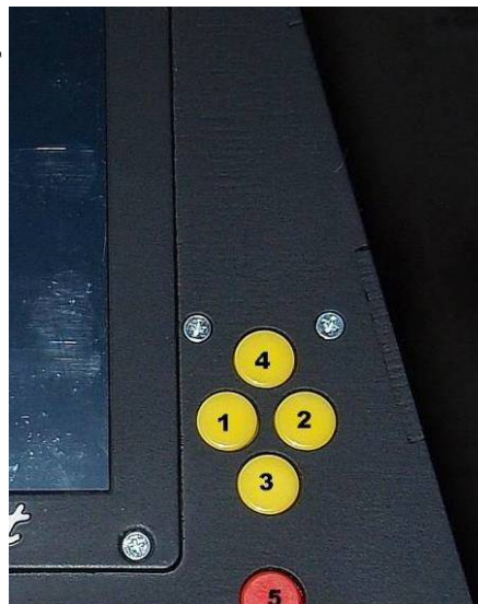
Figure 2 – Keypad (front panel) with 5 buttons to control the main machine functions
