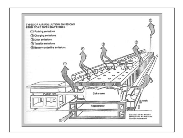
There are several sources of emissions from coke production facilities. Coal dust emissions occur as the coal is unloaded, crushed and transferred to the larry car. These emissions are not considered hazardous.
