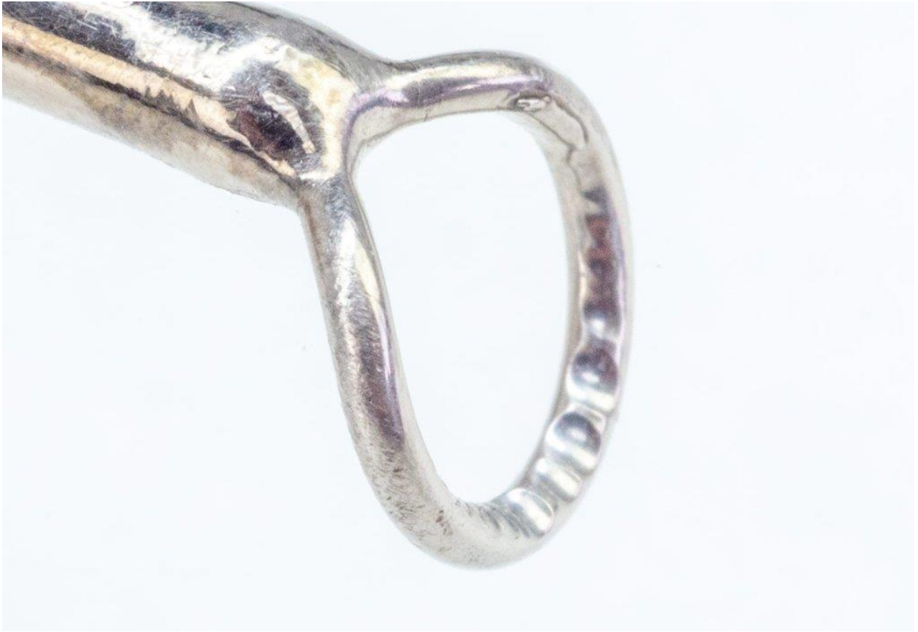
A badly grooved tip top. It's done a few miles and is showing it.
