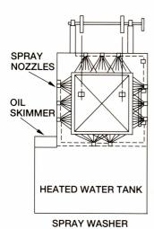
New 24"W x 36"D x 20"H multi-zone BeaverMatic unit combines temper furnace processing with a two chamber washer in one continous operation.
