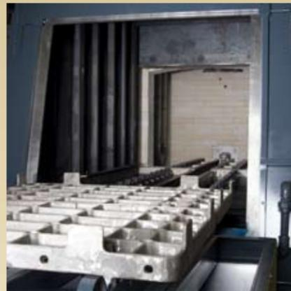
Atmosphere is circulated throughout the heating chamber by a belt-driven air-cooled alloy fan located in the roof of the furnace. The design reduces downtime and replacement costs, thus curtailing atmosphere gas and energy requirements.
