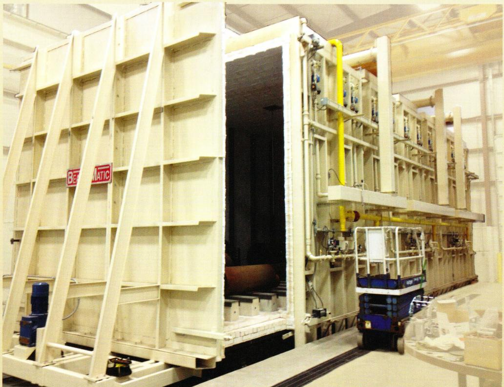
Carbottom Furnace capable of processing a 14 foot wide
