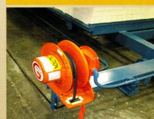
Car drive system with cable reel is required to drive the car in and out of the furnace for loading and unloading.
