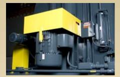
Large oil quench tanks provide the volume of oil required to meet specific needs. A double-decked elevator in the guench chamber facilitates recharging the furnace while a load is being quenched. Atmosphere quench chambers are optionally available.
