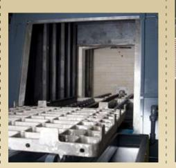
Atmosphere is circulated throughout the heating chamber by a belt-driven air-cooled alloy fan located in the roof of the furnace. The design reduces downtime and replacement costs, thus curtailing atmosphere gas and energy requirements.
