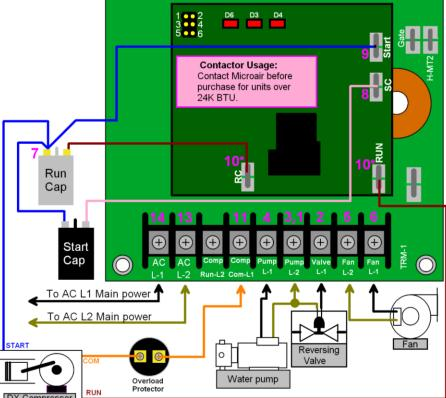
10\* Disconnect compressor "R" wire and connect to "RUN" terminal on EasyStart top board. Connect remaing wire from run capacitor to "RC" terminal on EasyStart top board.
