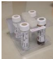
Volatiles for soils using a 5035 Kits:
