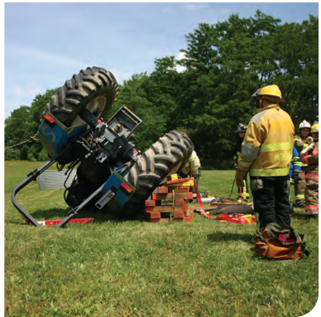
Figure 24-6: If necessary, call specialized personnel, such as the fire department, to stabilize and shut down heavy equipment.
