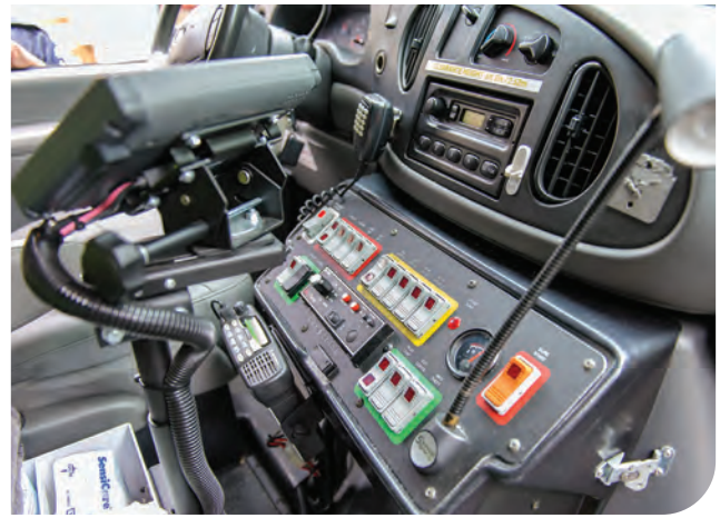
Figure 1–5: A radio communication system in an emergency vehicle.
