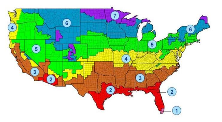
The Department of Energy recommends using different insulation levels based on regional climate zones to increase energy efficiency.
