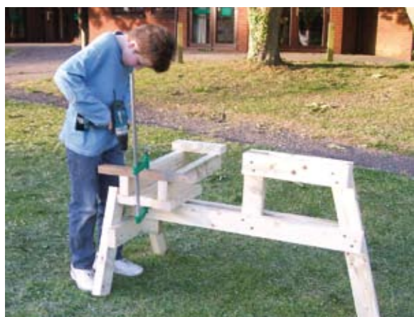
Stage 9: Fix the top bar and footrest to the arms.
