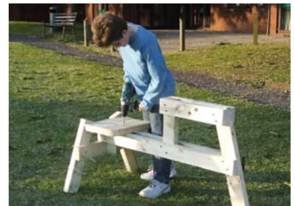
Stage 8: Fix the remaining seat sections.
