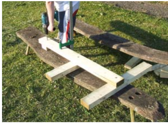
Stage 1: Fix a bed section to front leg, riser and spacer.
