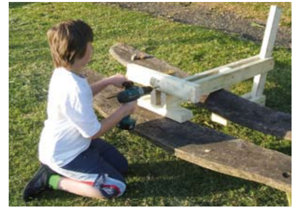
Stage 5: Fix the rear leg brace to the rear spacer.
