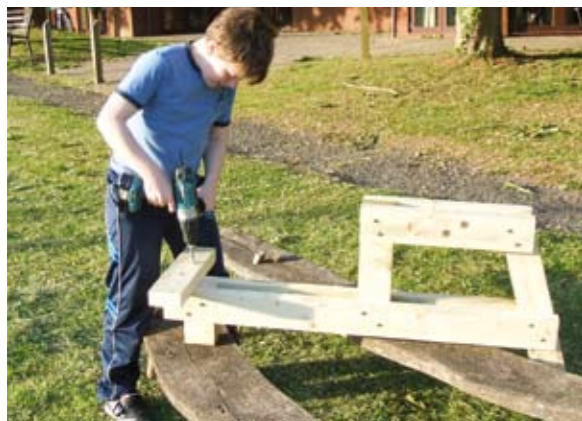
Stage 4: Fix the rear seat section.
