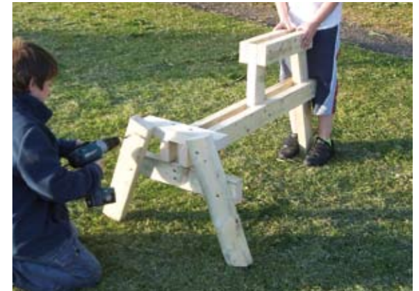
Stage 7: Fix the rear legs to the seat.
