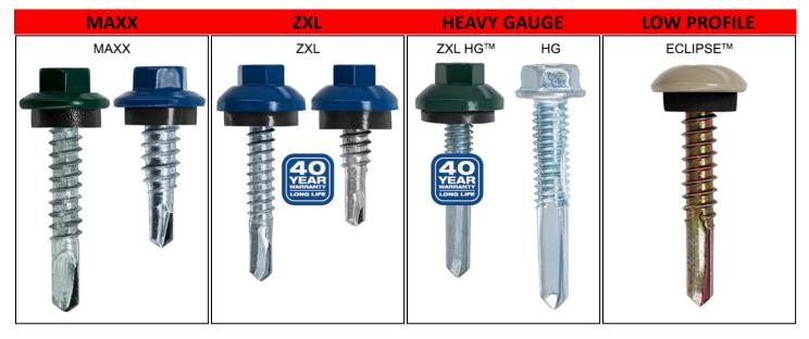
Fastener designed to attach metal roof and sidewall panels used in pre-engineered metal building applications. Included EPDM washer. Fastener designed to attach longlife metal roof panels such as GALVALUME that are used in preengineered metal building applications. Included EPDM washer. Metal to metal fasteners that selfdrill up to .500" steel thickness designed for maximum pull out strength. Included EPDM washer.
