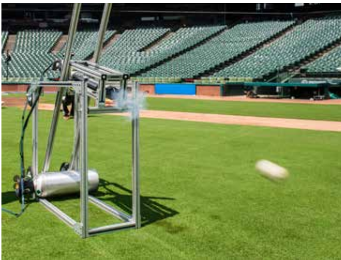
SHAW SPORTS TURF'S SIGNATURE BASEBALL CANNON LEADS THE WAY AS AN INNOVATIVE BENCHMARKING TECHNIQUE. WE TEST FIELDS WITH OPTIMAL PLAYABILITY TO RAISE THE BAR FOR OUR NEW GENERATION OF BASEBALL TURF, B1K.
