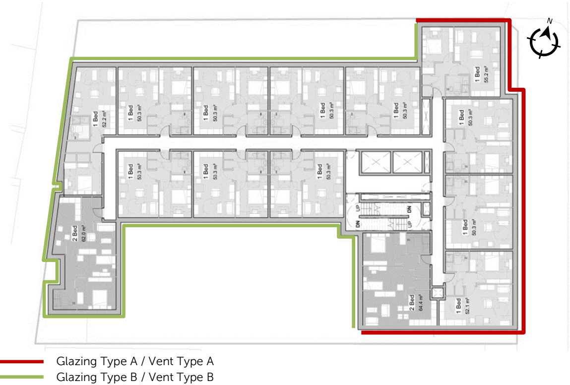
F4 Proposed First Floor Layout Illustrating Locations of Different Glazing and Ventilation Requirements
