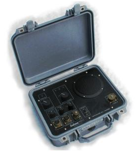
The Model 1020 — like all of Subsea's products — employs crystal-controlled single side band (SSB) ultrasonic techniques. Subsea's SSB technology provides distortion free transmissions and extended battery life. Users will enjoy clear communications even in strong currents or waters crowded with ships, wharf pilings, or debris and even while inside sunken ships, pipes or other enclosed areas. The Subsea Model 1020 is compatible with all other Subsea communications products.
