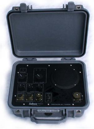
Advanced technology contributes to the superior quality and clarity of speech in the Scubaphone. Sophisticated electronic circuitry and filtering techniques are utilized to enhance speech clarity and reduce extraneous noises, thereby providing optimum clarity under adverse conditions. The Scubaphone Model 1080SX is a direct descendent of the Scubaphone Model 2000SX without the
