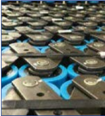
Escalator Step Chain
