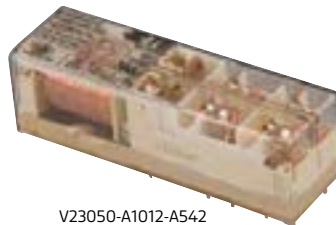
V23050-A1012-A542 Schrack Relay 12VDC, Safety, 4NO, DPST-NC, 250VAC, 8A
