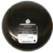
AB120 Alarm Bell, 120VAC .07 amp, 92 db
