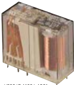
V23047-A1024-A501 Schrack Relay 24VDC 8230hm 6A DPDT 29 x 12.6 x 25.5mm
