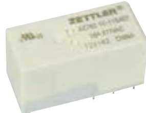
AZ762-1C-115AEF Relay 115VAC 8.1KOhm 16A SPDT
