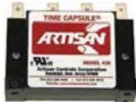
438115-5 Time Capsule Delay on make timer, 115VAC/DC 30 – 8,000 seconds MCE part # 27-01-0046
